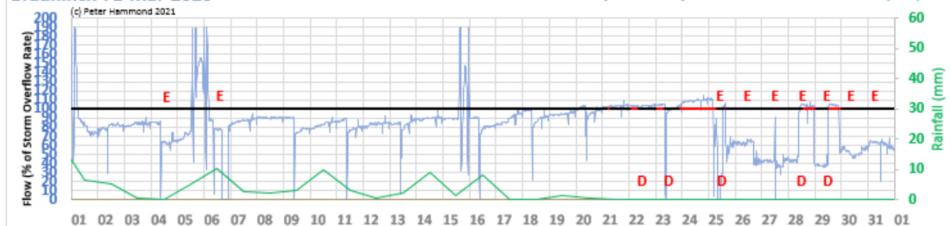
Figure 2: unpermitted spills of untreated sewage from Bradninch STW to the River Culm
