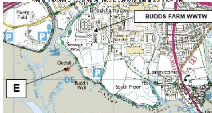
Figure 1: location of discharge outlets at Budd's Farm STW plus an extract of the EA permit for settled storm discharges into Langstone Harbour
