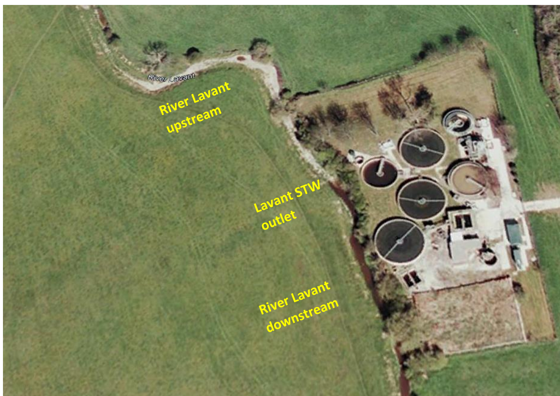
Figure 2: view of Lavant STW where riverbed is dry upstream and reddish-brown sewage effluent downstream
