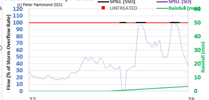
Figure 5: WASP believes there were at least 10 “early” spilling days (Jan 12,15-17,27; Mar 14-17, with Mar 25 and Apr 1 respectively losing 4.3 M litres and 2.4 M litres of untreated sewage (Mar 25 th )
