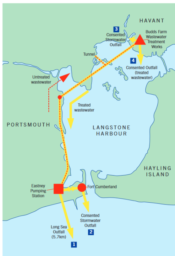
Figure 1: location of discharge outlets at Budd's Farm STW plus an extract of the EA permit for settled storm discharges into Langstone Harbour
