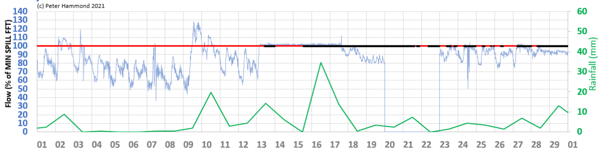
Figure 1: missing flow data coinciding with spills making compliance checking impossible (Jan 16-18 & Feb 20-22)
